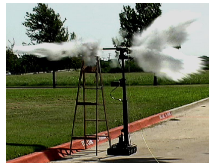
MURV-100 can fire recoilless disrupters at elevations up to 235cm (example: airplane overhead luggage bin) and down to ground level (example: pipe bomb). Disruptors fired here are Proparms 20mm Recoilless Units
