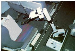
Optional turntable rotates either arm sideways for viewing, handling and disrupting
