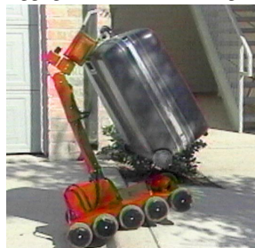
MURV-100 can pull airport luggage cart and lift 22.7kg
