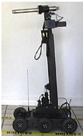
High-rise arm (above) and standard arm (right) are interchangeable
